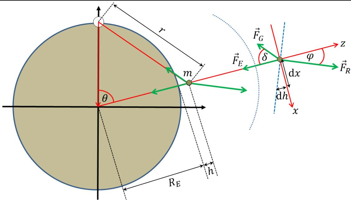
**Figure 3.S2** Same figure as above, but with the relevant forces depicted and showed again outside figure for clarity. The blue dotted line indicates the Earth surface. The blue dashed line indicates the local sea level, growing towards Greenland and decreasing towards the south pole.
