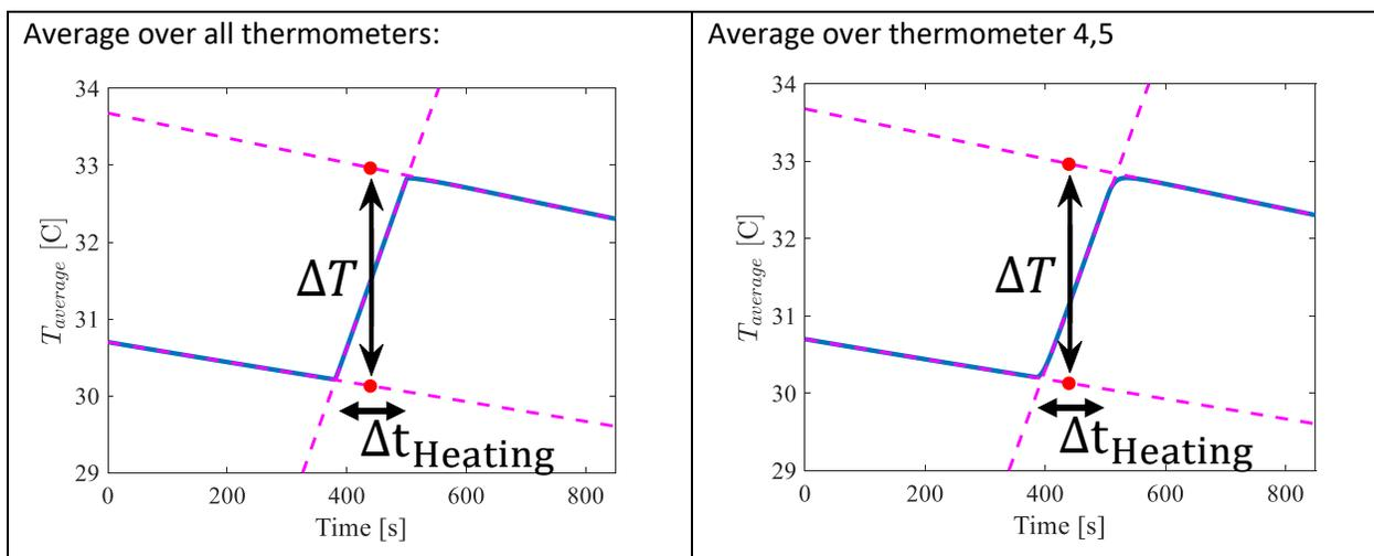
Both methods reproduce the heat conductivity within 1%,  $386 \left[ \frac{J}{kg \cdot K} \right]$ .
