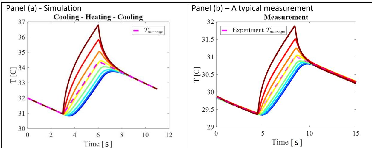
Panel (a) – a simulation of the cooling-heating-cooling cycle. Panel (b) – a typical cycle as measured in a real system. The different colors correspond to different thermometers.
